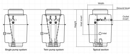
All pump chambers are available for dirty water (DW) or sewage (SW), in single pump (SP) and twin pump (TP) configurations.
